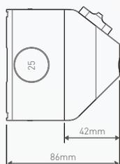
**SURFACE:** Featuring a hardwearing exterior, the surface mount option is our most versatile solution offering ample wiring space and 25mm conduit knock-out entries. Ideal for commercial use.
